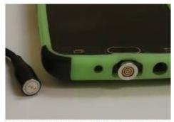
Photo 4: 4 wire Magnetic Data Cable and Adapter on Phone
